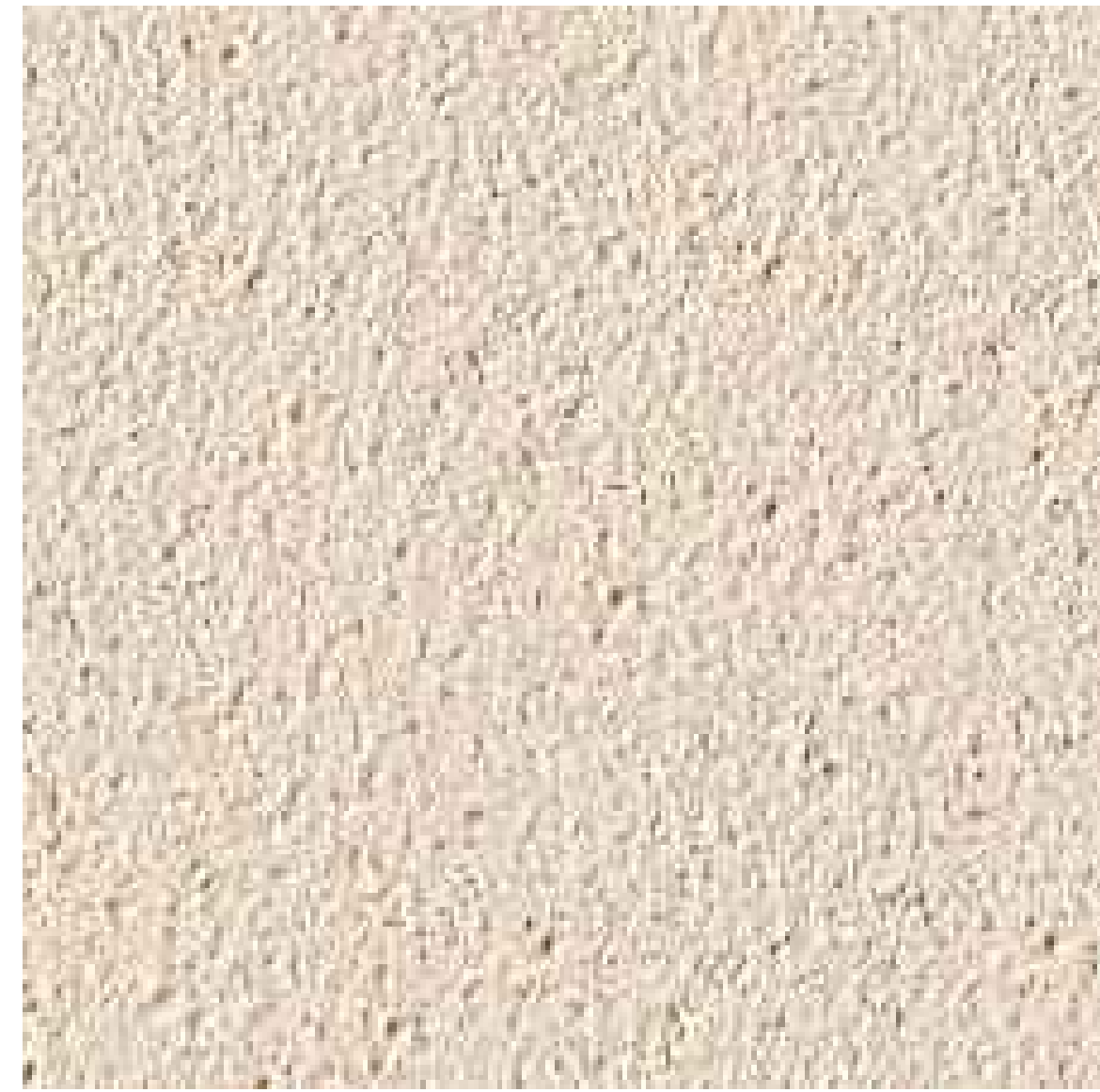
2 EXTERIOR CEMENT PLASTER LA HABRA - SAND FLOAT 20/30
